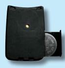
Carefully slide out battery holder and remove batteries. Install new batteries using the correct polarity. Use only CR-2325 or equivalent.
