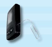
Press a paperclip into the tiny hole on the side of the unit and release. The unit restarts. Note: Reset the unit after battery replacement and when trouble shooting.
